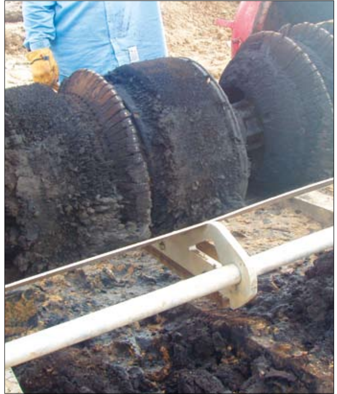
An effective pigging program will help prevent debris from building up in a pipeline and causing lost production and revenues.
